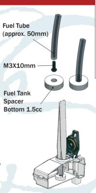
Using tweezers, push Fuel Tank Spacer onto the mounting pin
